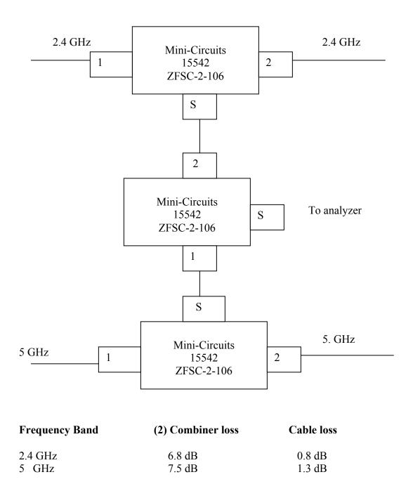
NOTE: Tests were performed with only one band (2.4 GHz or 5 GHz) operational at a time. The test set-up shown was employed as a matter of convenience, so that attachment to cardbus antenna ports would be made only once, minimizing wear and tear to connectors.
