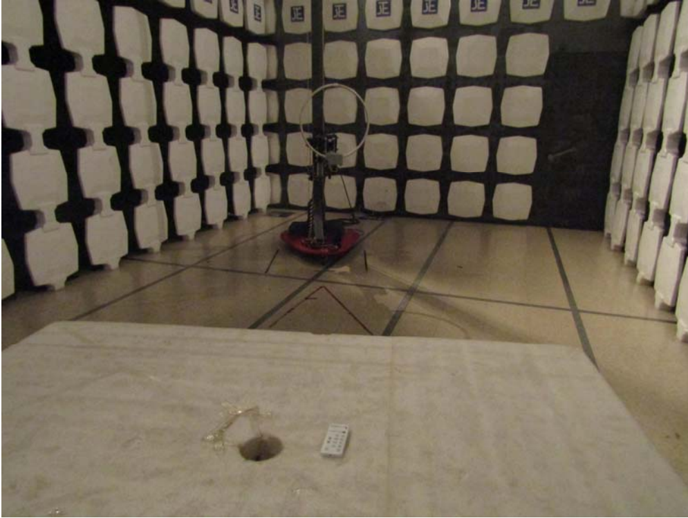
Measurement of Radiated Emission Test Set Up
