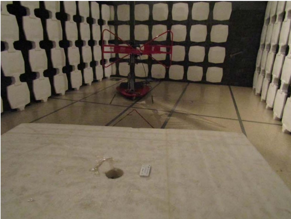
Measurement of Radiated Emission Test Set Up
