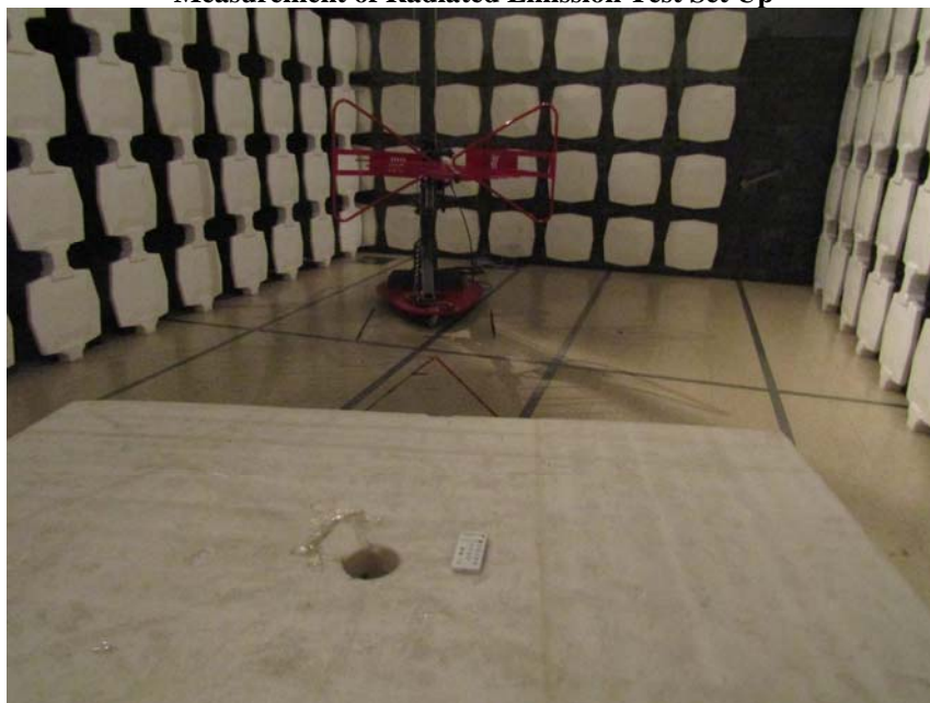
Measurement of Radiated Emission Test Set Up
