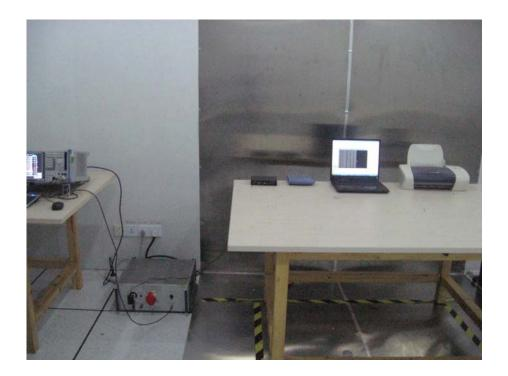
Radiation Emission Test Setup (30MHz to 1GHz)
