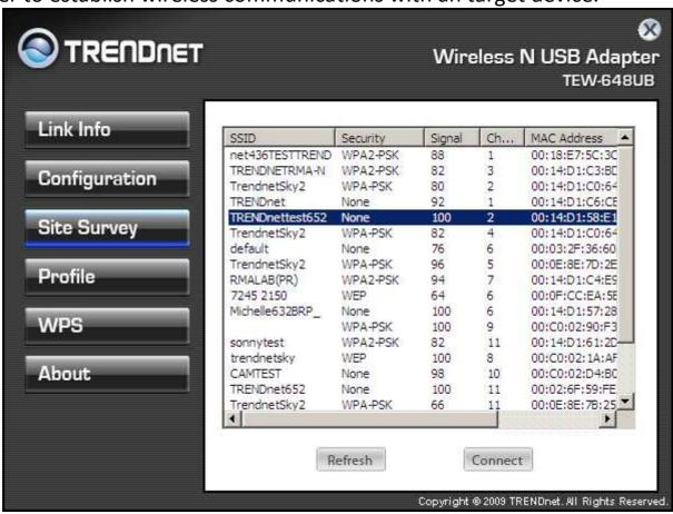
**Available Network** – displays the wireless networks (wireless clients, access points or routers) that are within range.
