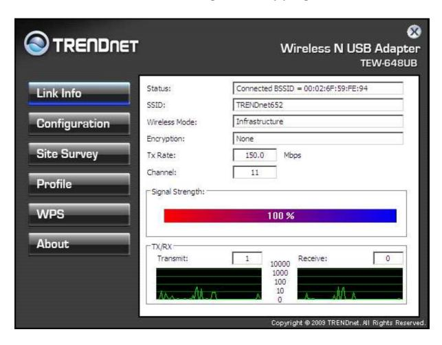
**Status:** Shows the associated BSSID (MAC address), which can be used to identify the wireless access point or router that you are connecting to.
