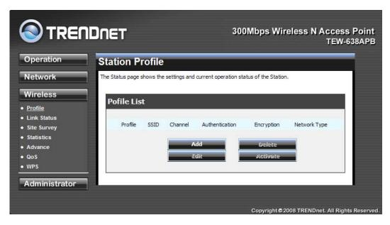
Configure the setting to connect to a wireless network, selection option for network type, SSID, and wireless security. The profile can be edited, deleted and made active from this option.
