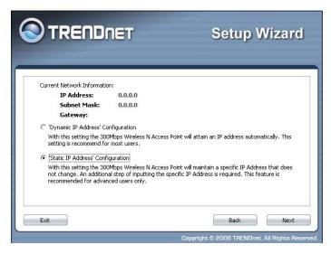
11. The default IP address is 192.168.10.100, you can choose to obtain network setting automatically, or set the IP address manually. After setting, click **Next** to complete it.
