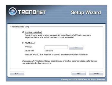
21. Use **PIN Method** and click **Select** to choice an AP SSID, and then click **Connect** button to make wireless connection.
