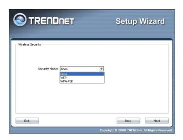
11. To use WEP security, select **WEP** and click **Next** button. Select **64-bit** or **128-bit** WEP key length, and enter your WEP key. For 64-bit encryption, enter 10 hexadecimal characters, For 128-bit encryption, enter 26 hexadecimal characters. Click **Next** to continue the setting.
