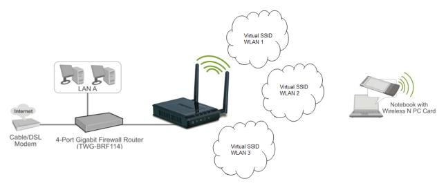
Multiple SSID (Virtual WLANs)
