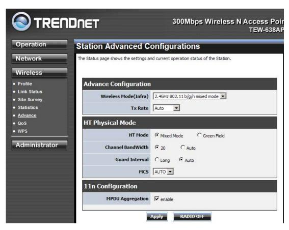
In **Advance Configuration**, select the **Wireless Mode** for the TEW-638APBto match the speed of the Access Point or wireless Router that will be connecting with. Select the following from the drop down list.
