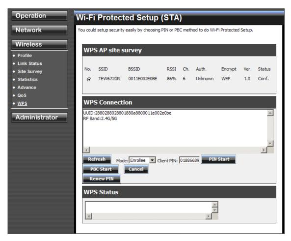
Two WPS modes can be selected – PIN & PBC. If PIN is selected, you should enter PIN code of your wireless client device to get wireless connection with this AP.
