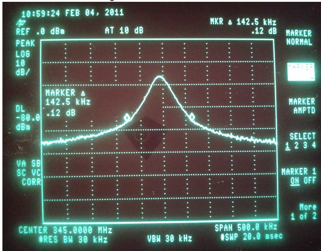
Bandwidth of the modulated signal is 142.5 kHz
