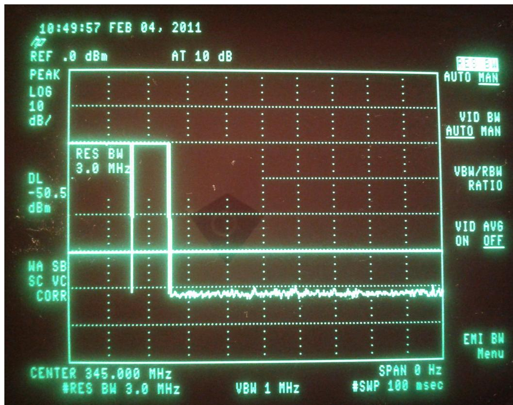
Plot below shows an expanded view of the transmitted packet.
