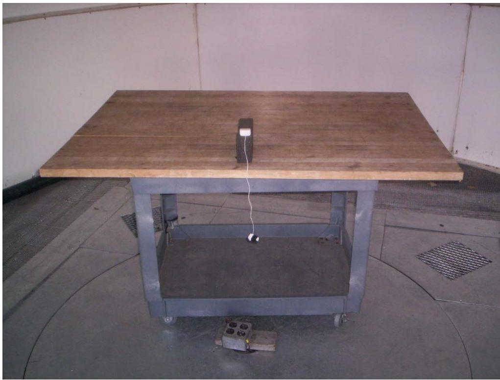
**Appendix C : Block Diagram of Test Setups****Test Site For Radiated Emissions**
