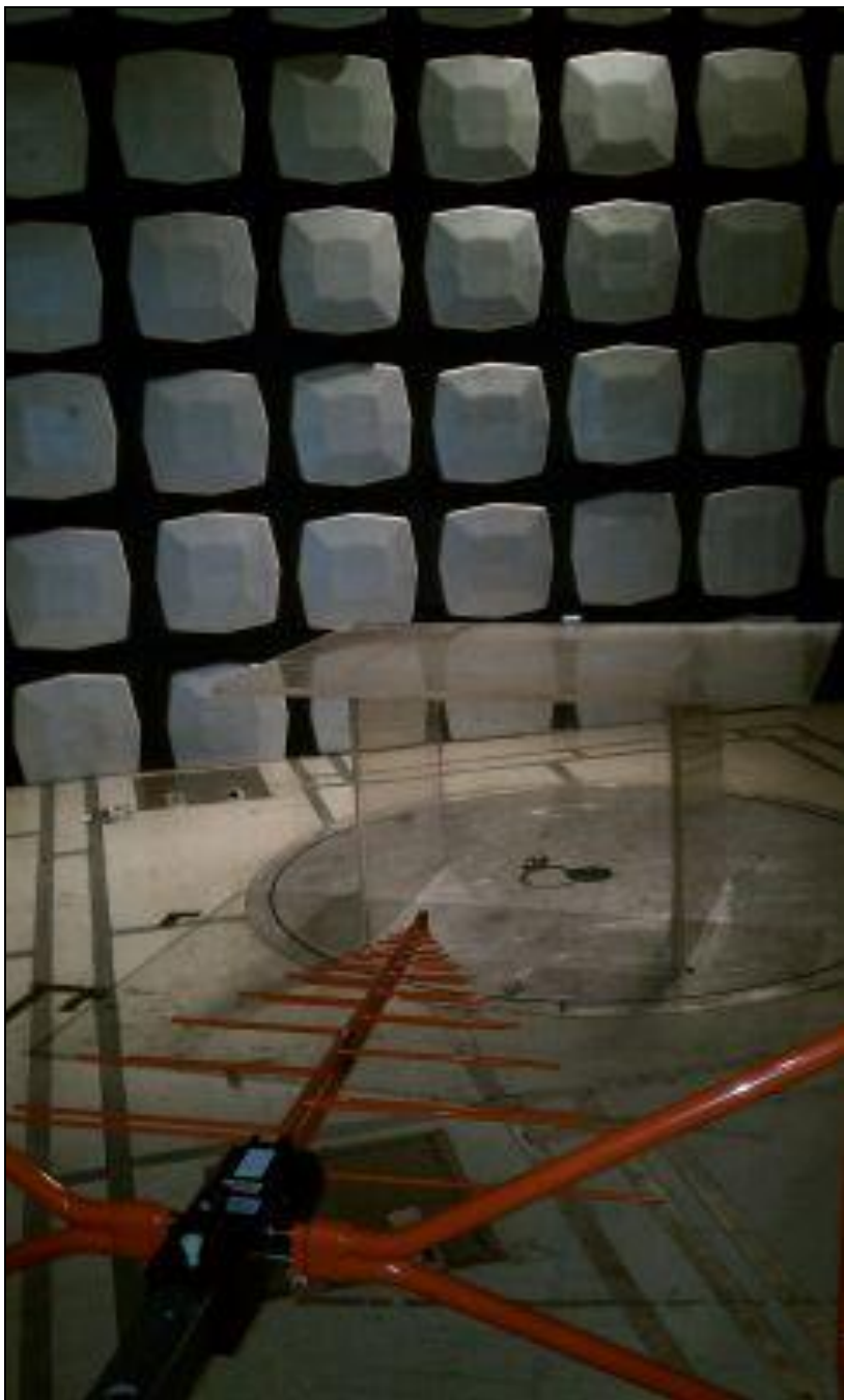
Photograph 2. Radiated Emissions, Test Setup, 30 MHz – 1 GHz
