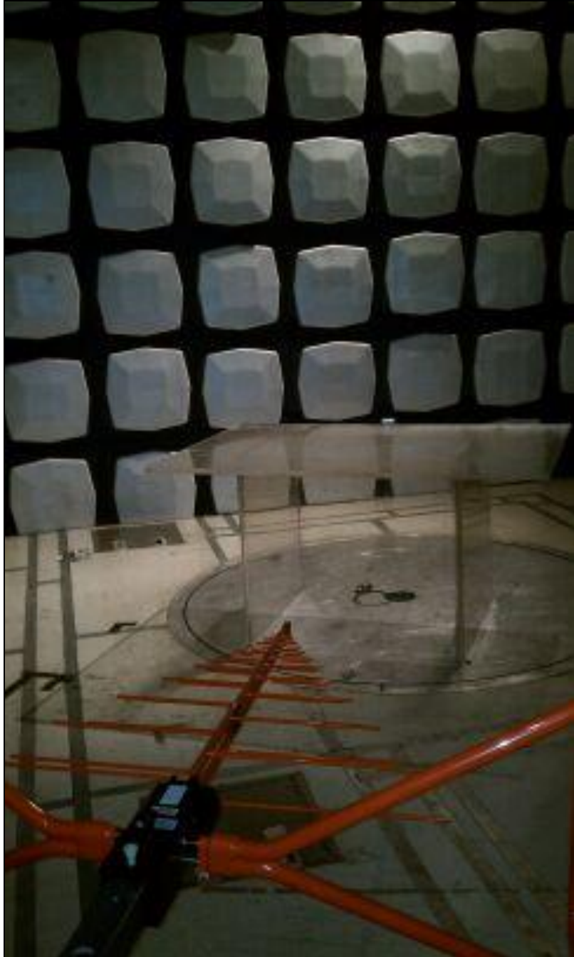
Photograph 3. Radiated Spurious Emissions, Test Setup, 30 MHz – 1 GHz
