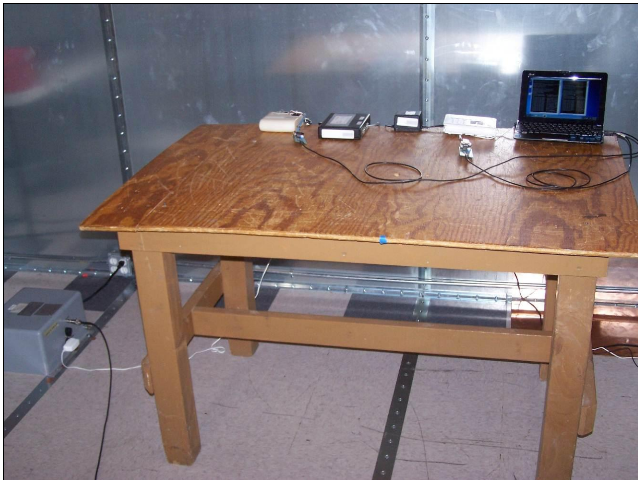
Photograph 4. Conducted Emissions, 15.207(a), Test Setup
