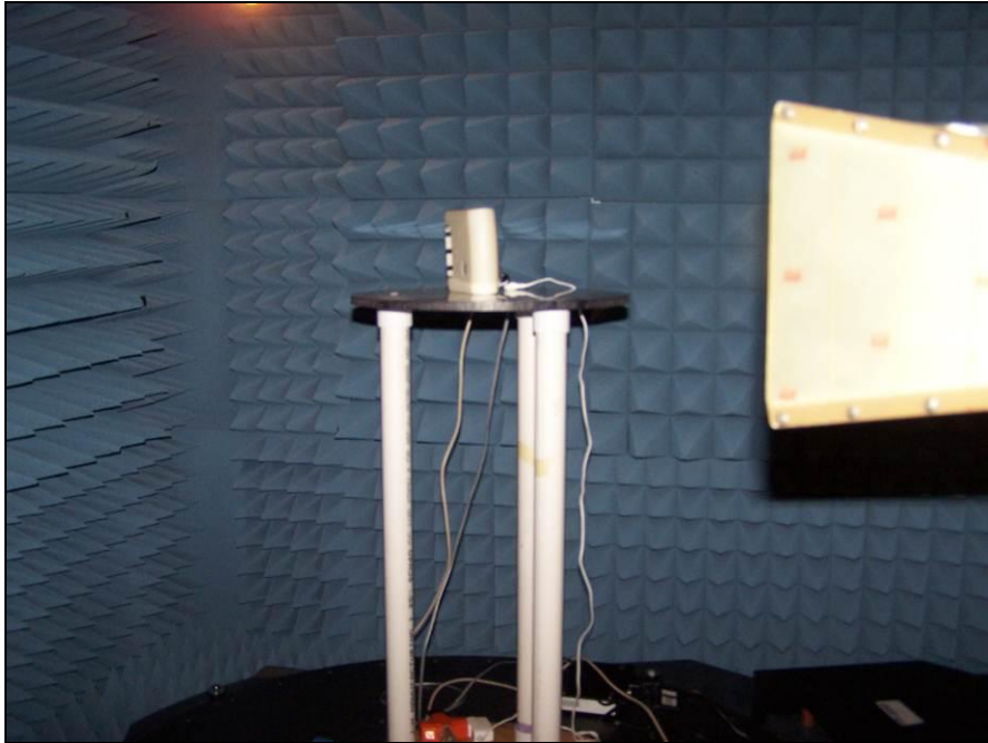
Photograph 5. Radiated Spurious Emissions, Test Setup
