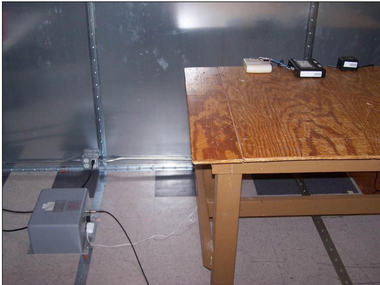
Photograph 2. Conducted Emissions, Test Setup without Radio
