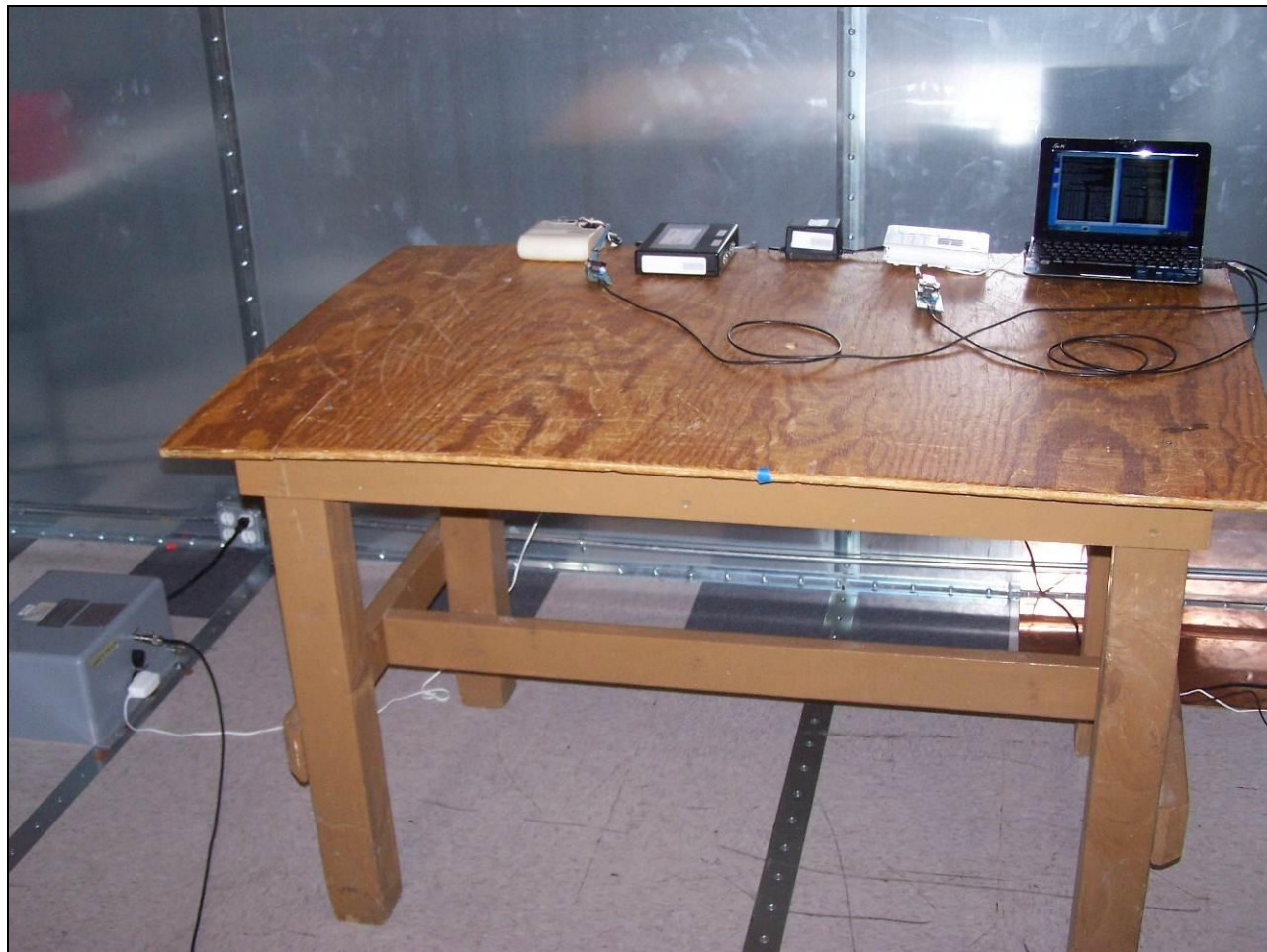
Photograph 4. Conducted Emissions, 15.207(a), Test Setup
