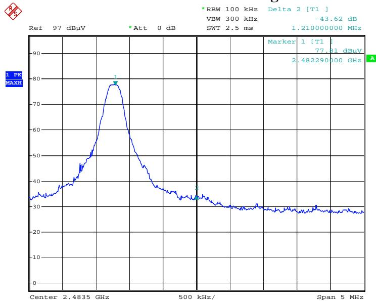
Measured Field Strength for High Channel in 1 MHz RBW = 114.7 dBμV/m
