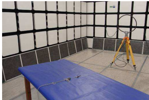
Set up of Radiated emission test (ANTENNOVA antenna)
