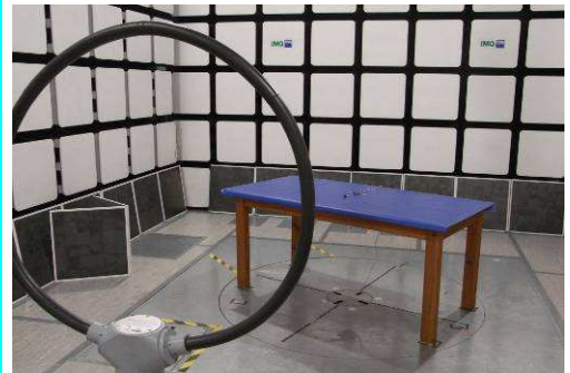
Set up of Radiated emission test (ANTENNOVA antenna)
