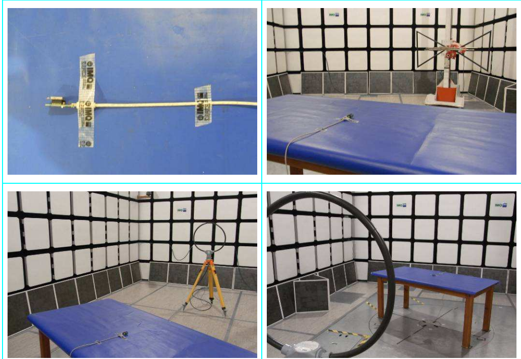
Set up of Radiated emission test (RAINSUN antenna)
