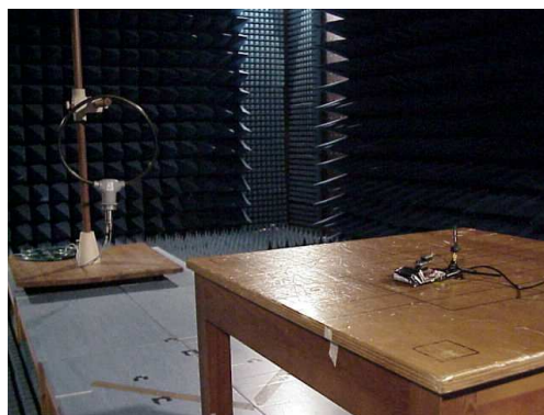
Set up of Radiated emission test (ANTENOVA antenna)
