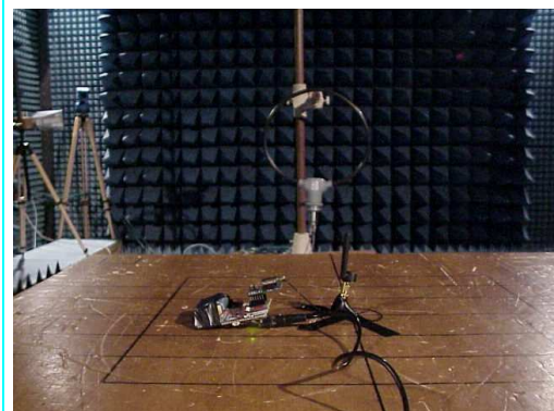
Set up of Radiated emission test (ANTENOVA antenna)
