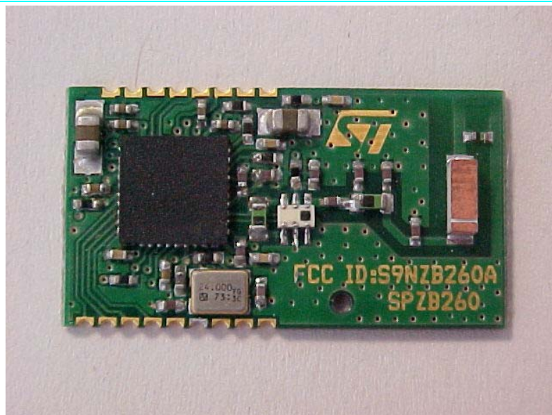
Radio module with MURATA antenna
