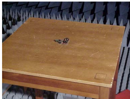
Set up of Radiated emission test
