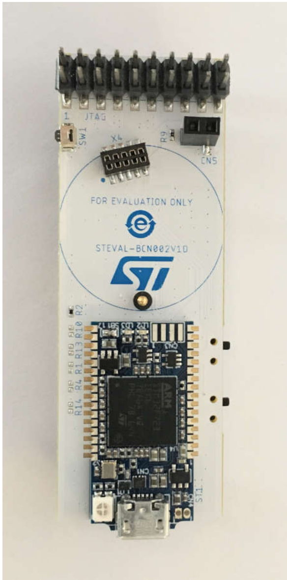
Figure 7: STEVAL-BCN002v1D top view with and without STLinkv3
