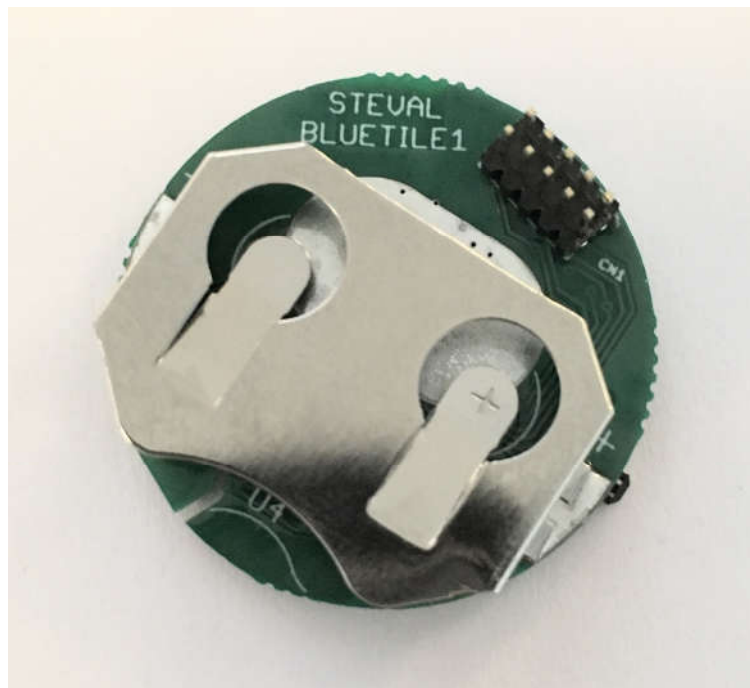
Figure 5: STEVAL-BCN002v1 bottom view with battery holder
