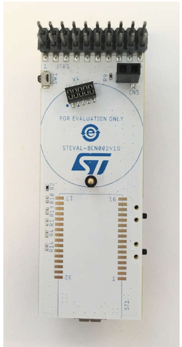
Figure 7: STEVAL-BCN002v1D top view with and without STLinkv3
