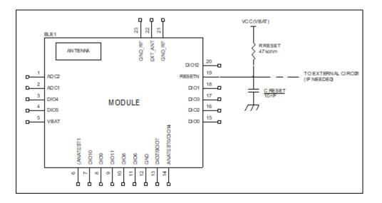
If reset pin is controlled by an external host, there is no need to have RC circuit on the RESETn line.
