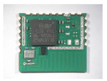
Photograph showing a BLUENRG-M2SP, with shield removed.
