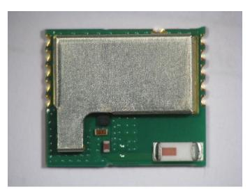
Photograph showing a generic BLUENRG-M2SP, covered by metallic shield.
