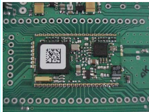
Equipment under test identification: Test jig + Radio module
