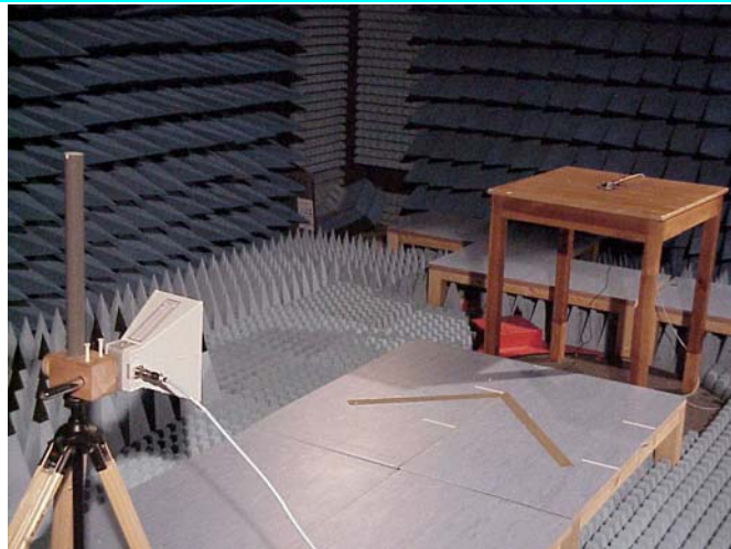
Set up of Conduced emission test
