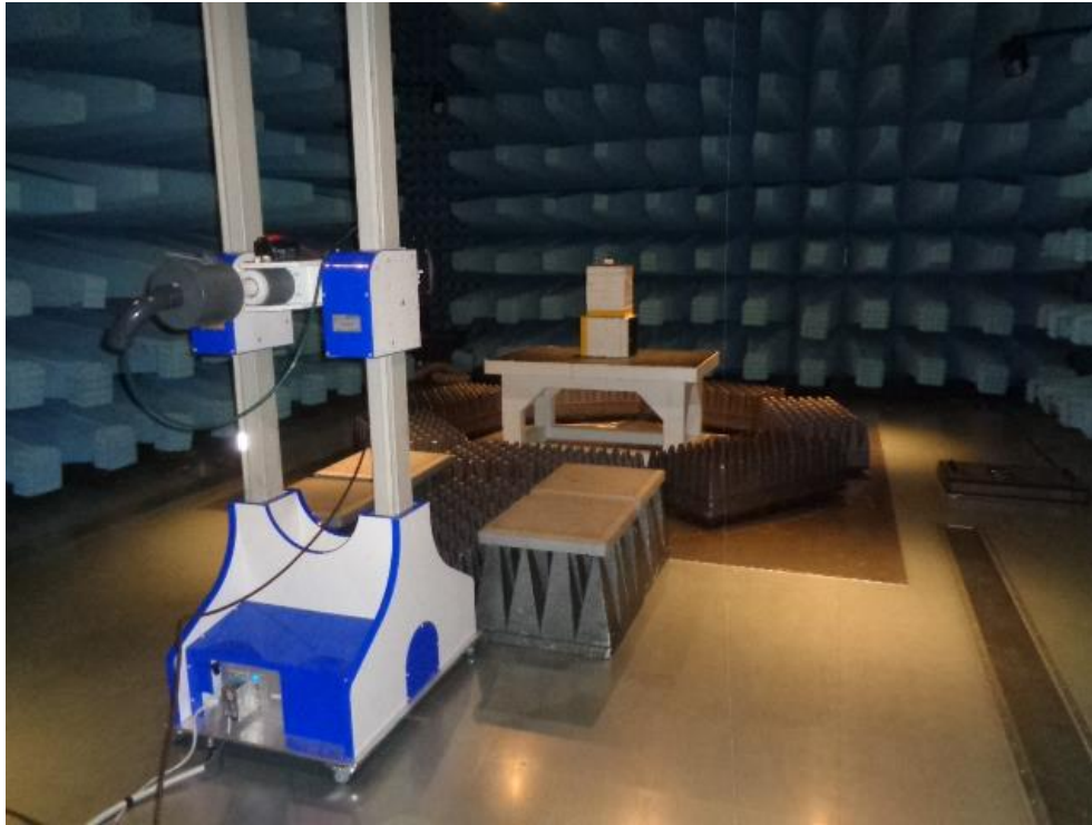
Figure 9.1-2: Radiated emissions set-up for frequencies above 1 GHz
