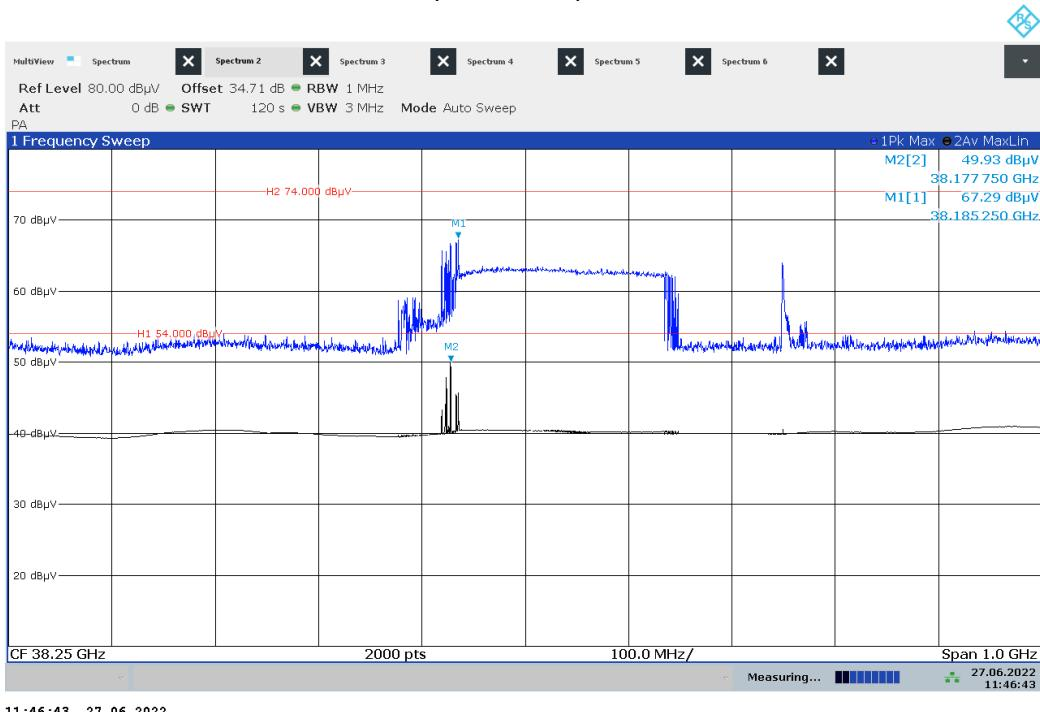
Plot no. 62: radiated emissions 26.5 GHz – 40 GHz, high speed mode, polarization vertical / horizontal
