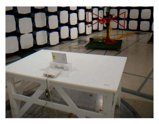
16.10 Radiated Emission above 1 GHz Rear View (5 dBi Patch Antenna)
