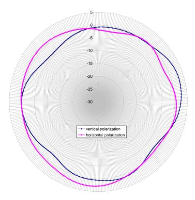
Conclusion: Antenna patterns were measured in an anechoic chamber and it was determined that the highest gain for antenna in 2.4GHz band was 3dBi.
