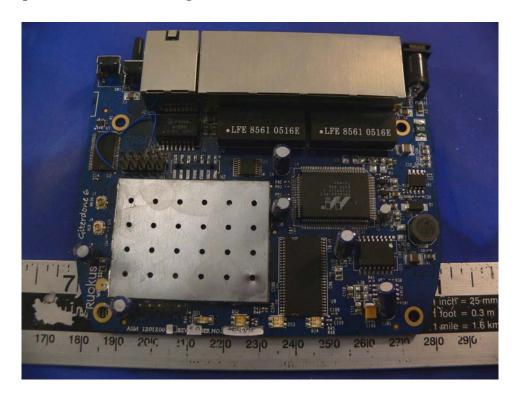
**EUT – Component View without shielding**
