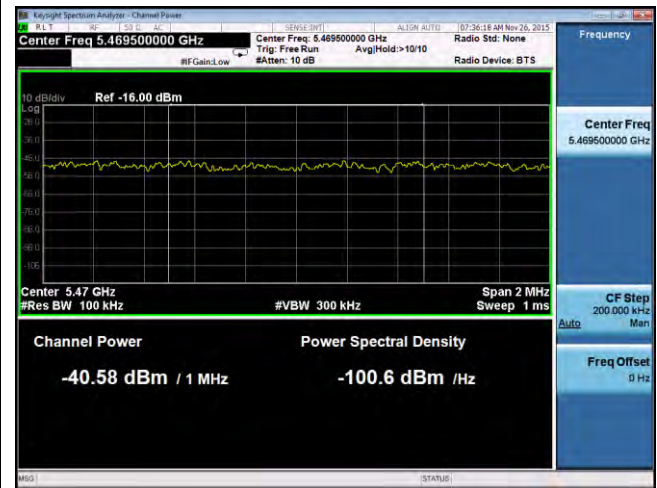
Band Edge -802.11ac-80M-5530M-chain2 (Left)
