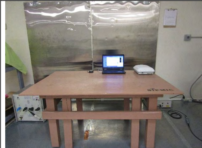
AC Line Conducted Emissions – PoE – Front View
