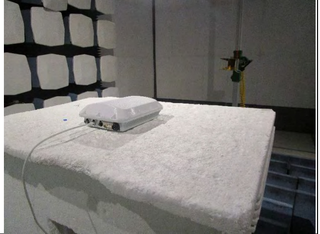
Radiated Emissions (>1GHz) – Rear View
