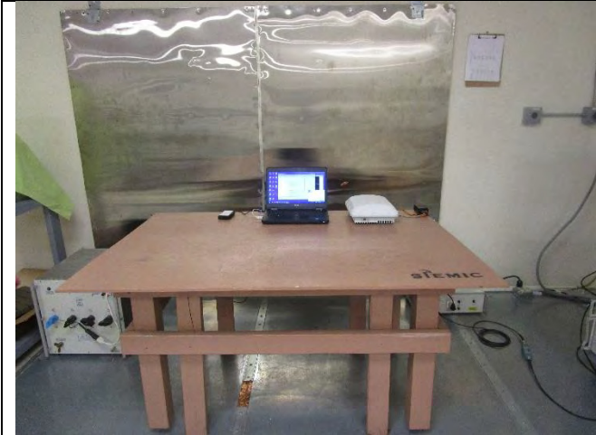
AC Line Conducted Emissions – AC Power – Front View
