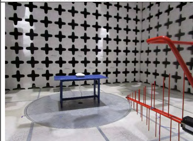
Radiated Emissions (<1GHz) – Front View
