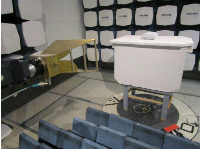
Radiated Emissions (>1GHz) – Front View
