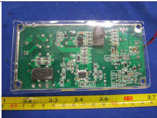
EUT Internal Power Distributor – Solder View
