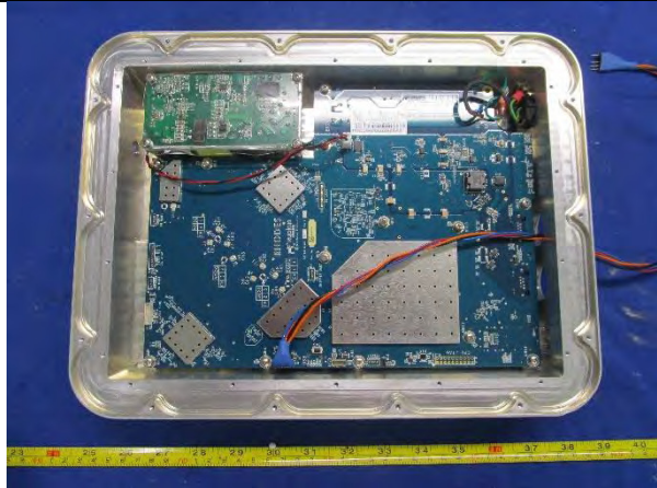
EUT Open Chassis with Antenna Board Removed
