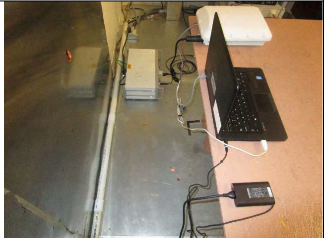
AC Line Conducted Emissions – PoE – Rear View
