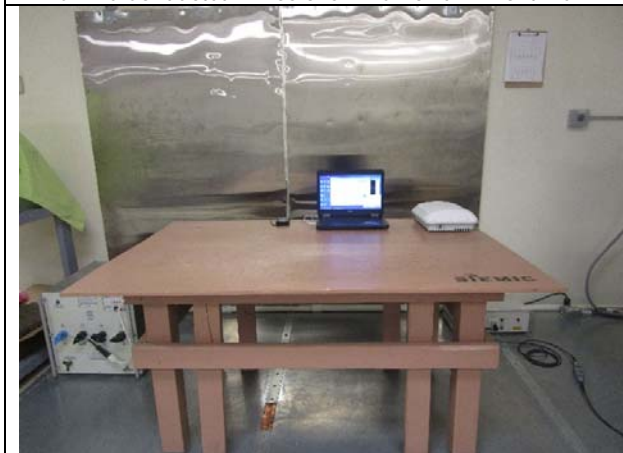
AC Line Conducted Emissions – PoE – Front View
