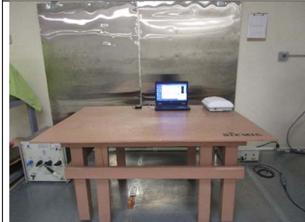
AC Line Conducted Emissions – PoE – Front View
