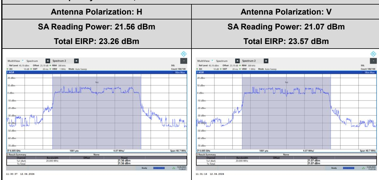
**SP AP Mode Max. EIRP Limit 33.84 dBm****DUT Center Frequency 6295 MHz, Bandwidth 20 MHz**
