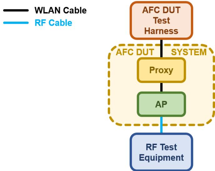
Proxy representing one Standard Power Access Points Test Setup
