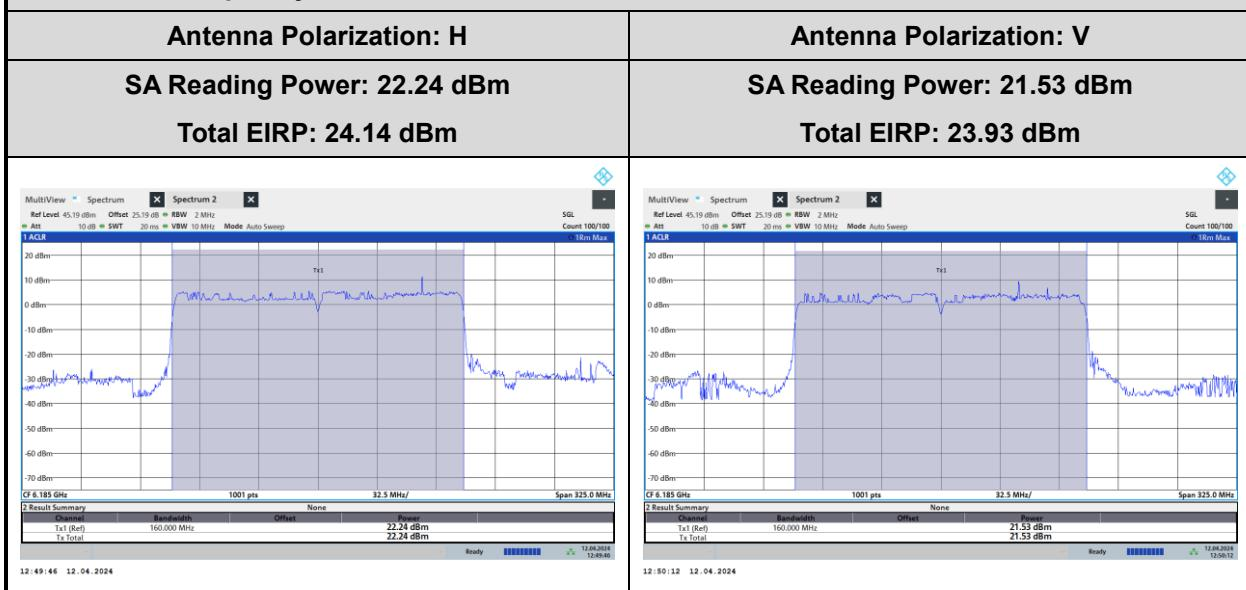
**SP AP Mode Max. EIRP Limit 30.84 dBm****DUT Center Frequency 6025 MHz, Bandwidth 160 MHz**
