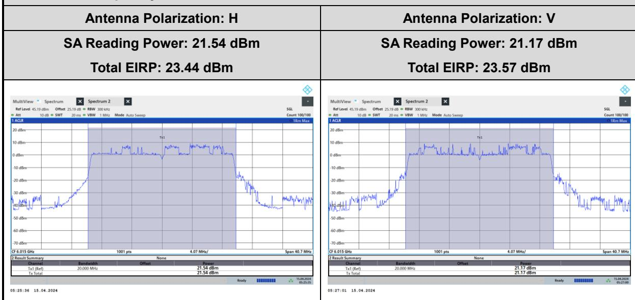
**SP AP Mode Max. EIRP Limit 34.03 dBm****DUT Center Frequency 6215 MHz, Bandwidth 20 MHz**
