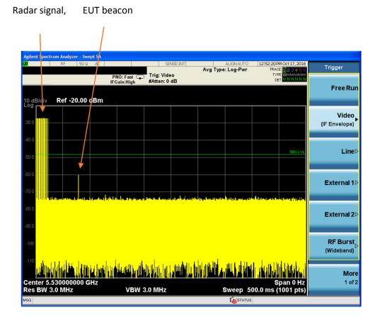
EUT have stream before radar signal detect.
