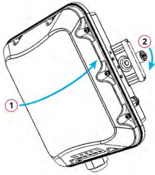
FIGURE 7 Attaching the Mounting Bracket to the AP
