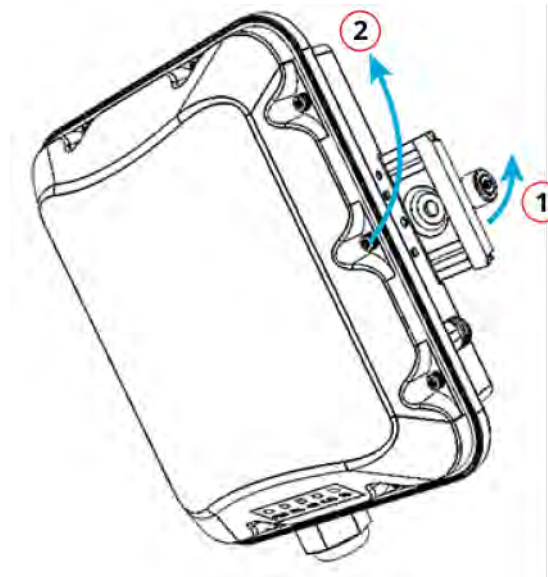
FIGURE 4 Removing the Mounting Bracket
