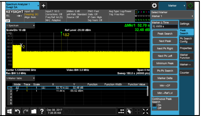
Radar at beginning of CAC – VHT80 – 5530MHz
