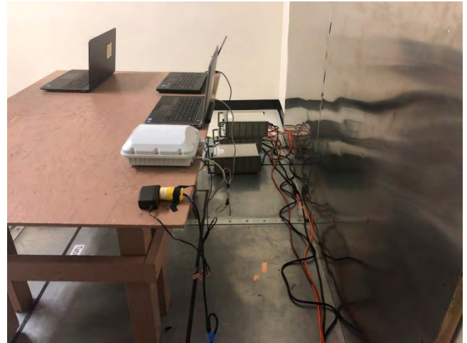
Conducted Emissions - Power Supply Mode – Rear View
