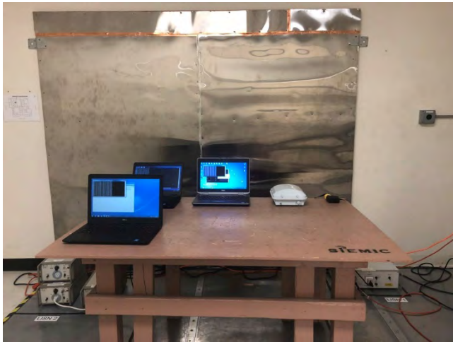
Conducted Emissions - Power Supply Mode – Front View
