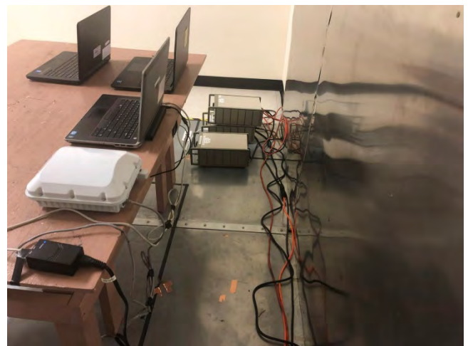
Conducted Emissions - P.O.E Mode – Rear View
