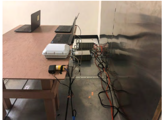
Conducted Emissions - Power Supply Mode – Rear View
