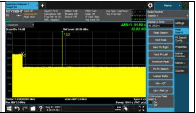
Radar at beginning of CAC – VHT80 – 5530MHz
