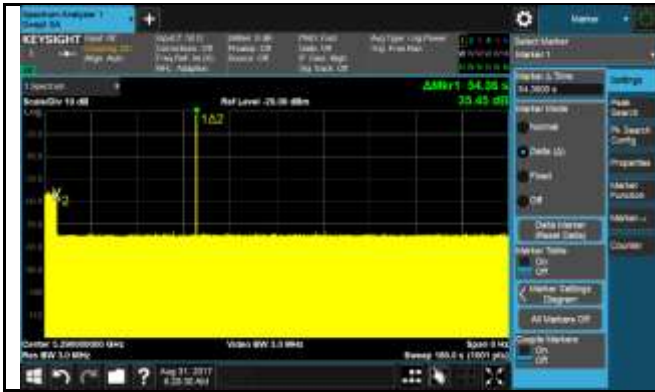
Radar at beginning of CAC – VHT80 – 5290MHz
