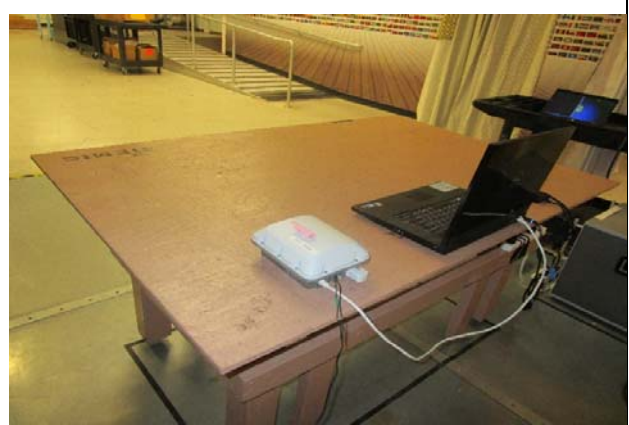
Conducted Emissions - Power Supply Mode – Rear View
