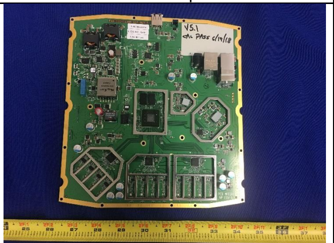
Main Board cover off- top view
