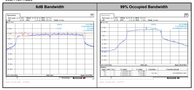
Note: The occupied channel bandwidth is maintained within the band of operation for all of the modulations.
