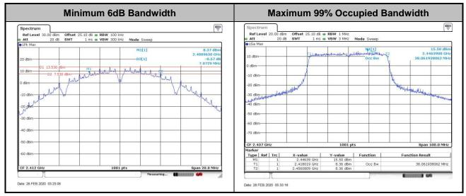
Note: The occupied channel bandwidth is maintained within the band of operation for all of the modulations.
