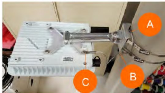
FIGURE 13 Attaching the Security Cable
