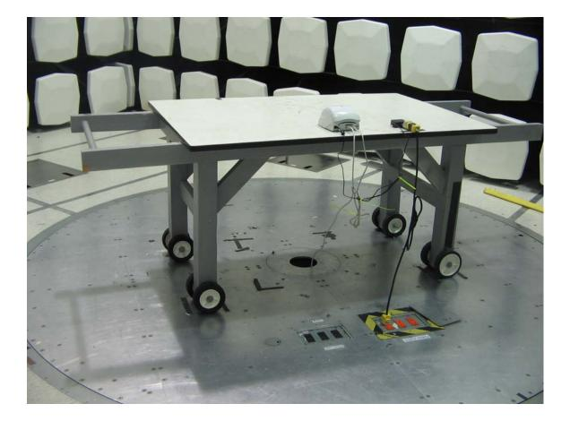
Radiated Emissions Test Configuration Photographs
