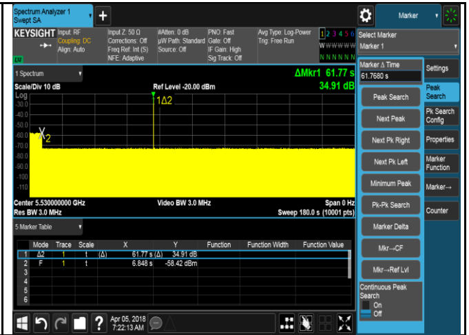
Radar at beginning of CAC – VHT80 – 5530MHz
