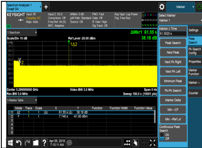
Radar at beginning of CAC – VHT80 – 5290MHz
