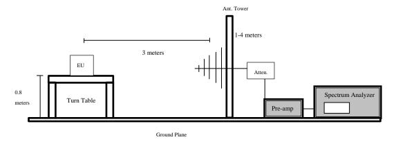
Test Setup for Above 1 GHz at 3 meters
