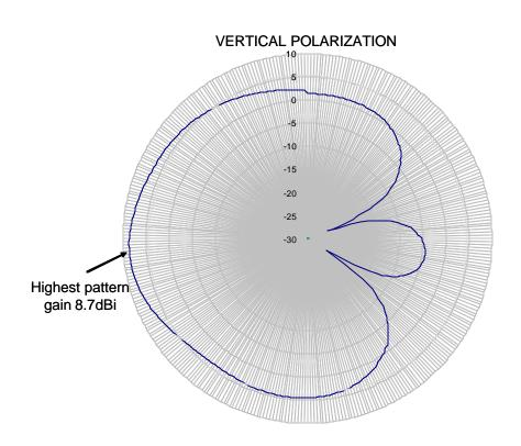
Each polarization on the antenna is capable of 64 different element combinations with horizontal polarization peak gain of 6.5dBi and vertical polarization peak gain of 8.7dBi.
