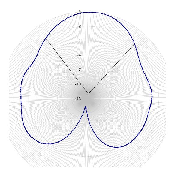
Conclusion: Antenna patterns were measured in an anechoic chamber and it was determined that the highest gain for all possible antenna patterns was 5dBi. HPBW is 71 degrees
