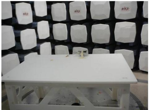
14.2 Radiated Emission below 1 GHz Rear View
