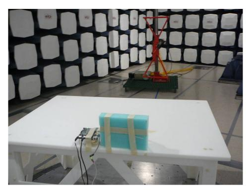
12.6 Radiated Emission above 1 GHz Rear View @15 dBi Antenna
