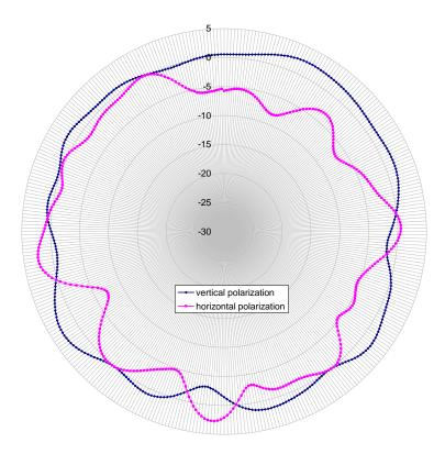
Conclusion: Antenna patterns were measured in an anechoic chamber and it was determined that the highest gain for both 2.4GHz and 5GHz antennas was 3dBi.
