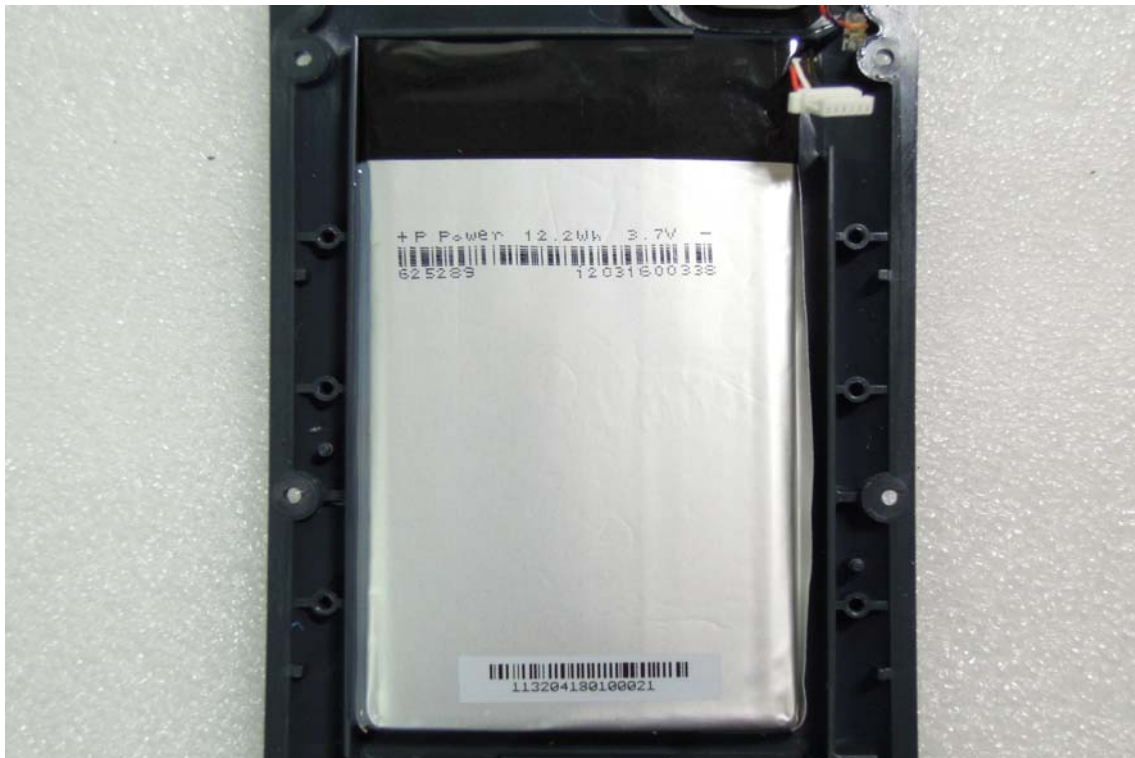
Battery (Model No.: S11GD103A, Supplier: LICO)
