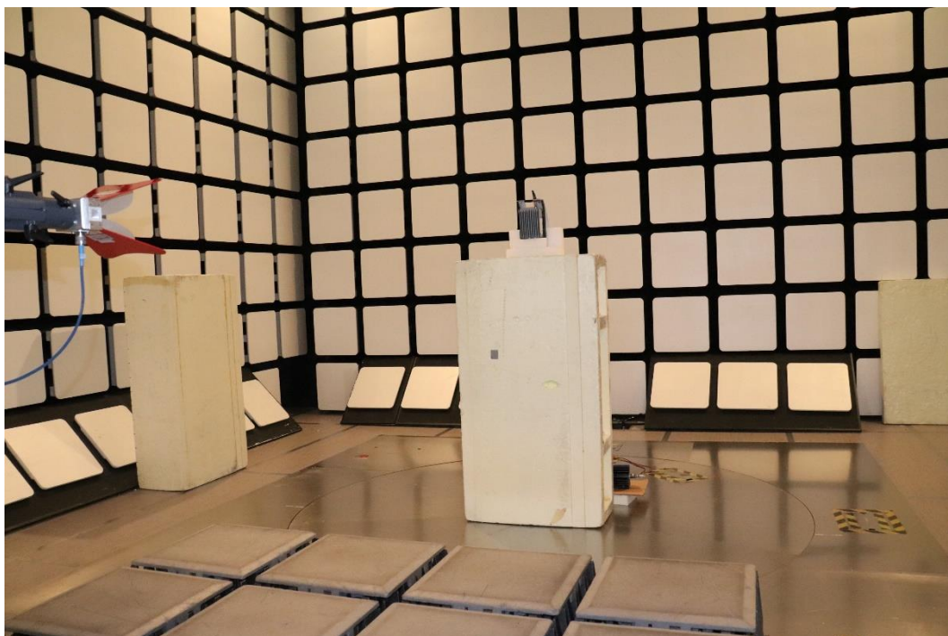
Photograph 6: Radiated emission test setup 1 – 5 GHz
